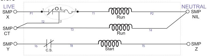
The RED and BLUE wires of the Solid State Start Switch take the place of the mechanical start switch.
